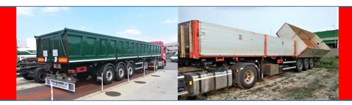
62 - Double tank double sided tipper semitrailers with aluminum sides
